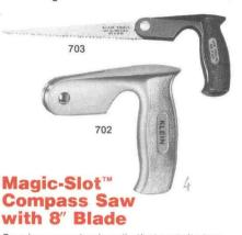
Saw has oversize handle that permits twohand use. Magic-Slot design allows fast blade changing without removing thumbscrew. Handle is strong, lightweight diecast zinc with blue finish, contoured for comfort. Blade is tough, high-quality carbon steel, 8" (203 mm) long, with 10 teeth per inch for general-purpose use. Replacement blade (No. 706) and handle (No. 702) can be ordered separately.
